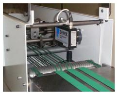
Batch count accuracy is assured by the laser sensor mounted downstream of the product bad-copy divert gate.
