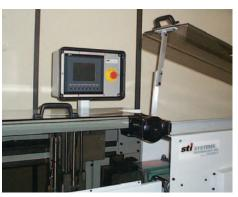
Simple touch screen operator controls assure easy make-ready and accessible process information.
